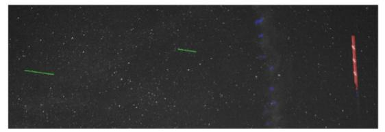
Figure 7: LEO objects detection. Sample result. Objects detection and automatic classification: two LEO objects (left) identified by the green colour, irrelevant objects identified by blue (right) and an airplane identified by red (right).
